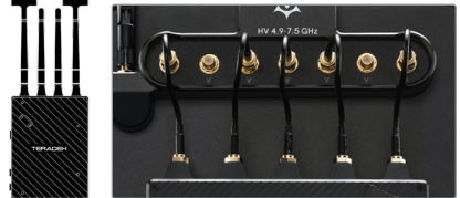
H+V antenna TX and RX configuration
